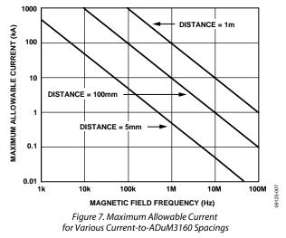
Note that, at combinations of strong magnetic field and high frequency, any loops formed by printed circuit board traces may induce error voltages sufficiently large enough to trigger the thresholds of succeeding circuitry. Care should be taken in the layout of such traces to avoid this possibility.
